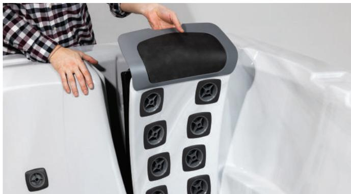
**ATTENTION :** LA POIGNÉE SITUÉE À L'ARRIÈRE DE L'APPUI-TÊTE DU JETPAK DOIT ÊTRE UTILISÉE POUR MANIPULER LE JETPAK (COMME INDIQUÉ). LA PRESSION APPLIQUÉE SUR LA PLAQUE AVANT EN ACRYLIQUE POUR LE RETRAIT, LE REMPLACEMENT OU LA MANUTENTION PEUT ENDOMMAGER LE JETPAK ET ANNULER LA GARANTIE.
