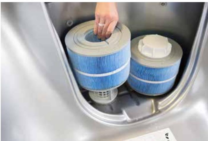
**Step 4:** Using a garden hose with a nozzle or other high-pressure device, clean cartridge(s). Work first from the inside, top to bottom on each pleat then from the outside, top to bottom on each pleat.
