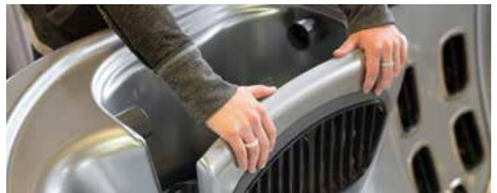
**Step 3:** Remove the pleated cartridge(s) by turning the filter core cap(s) counter clockwise then sliding the cartridge(s) upward from the filter core.
