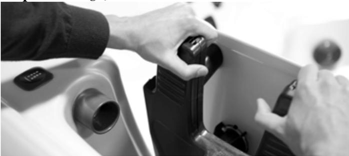
**Step 5:** Lower the manifold of the new JetPak carefully as to align the lower valve assembly and gasket into the bulkhead fitting. Apply pressure downward as you move the JetPak manifold until the manifold is secured in the wall clip assembly .
