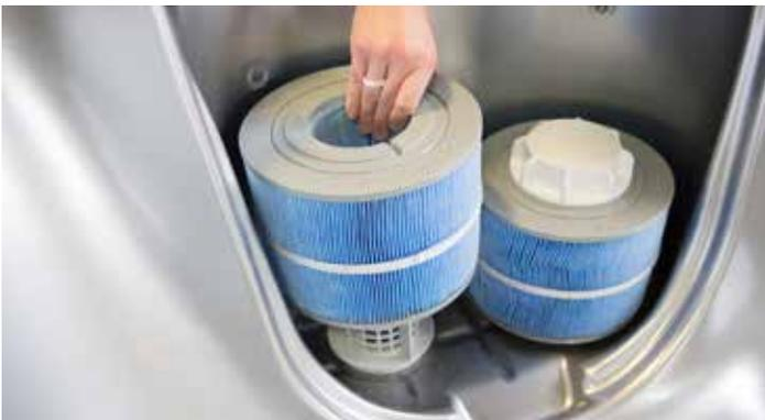
**Step 4:** Using a garden hose with a nozzle or other high-pressure device, clean cartridge(s). Work first from the inside, top to bottom on each pleat then from the outside, top to bottom on each pleat.
